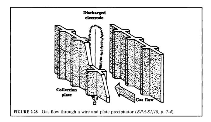
Migration velocity: Once the particle is charged, it migrates toward the grounded collection electrode. An indicator of particle movement toward the collection electrode is denoted by the symbol w and is called the particle migration velocity or drift velocity. The migration velocity parameter represents the collectability of the particle within the confines of a specific collector. The migration velocity can be expressed in terms of
